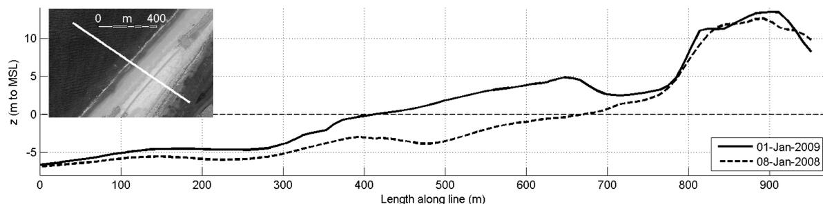
Figure 1. Two altitude profiles: after and before the construction of the new dune strip.
