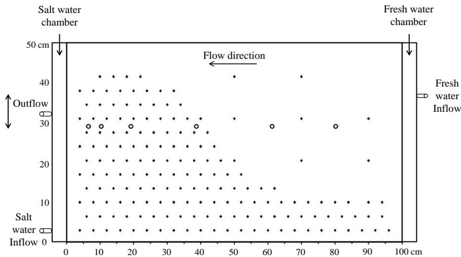
**Figure 1.** A schematic figure of the laboratory system. The black dots represent the location of the electrodes and the circles represent the location of the piezometers.
