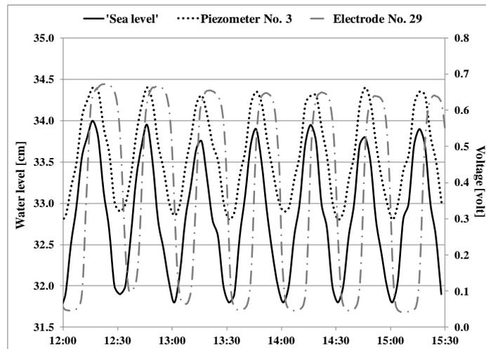
**Figure 2.** Preliminary results from the laboratory experiment. The groundwater level (dotted line) reacts immediately to 'sea level' fluctuations (solid line), while the FSI (grey dashed line) has a significance time-lag.
