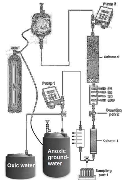
**FIG. 3.** A unique ASR column setup, showing reservoirs of oxic tap water and (deeply) anoxic groundwater, column 1 simulating the ASR proximal aquifer zone, and column 2 simulating the remote buffer zone.
