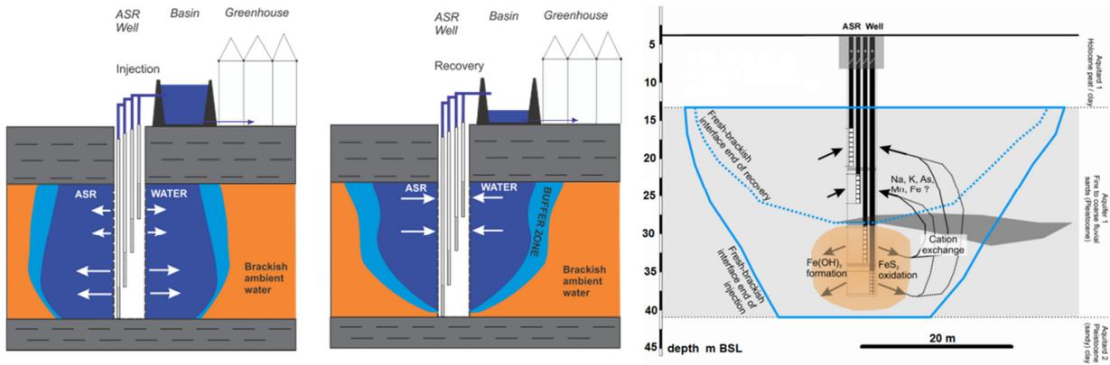
**FIG. 1.** Left and middle: Use of multiple partially penetrating ASR well for significant improvement of freshwater recovery from a confined brackish aquifer in coastal Netherlands. Right: Shift in position of the fresh water bubble after injection and after recovery, with important hydrogeochemical processes and zones.
