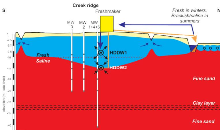
**FIG. 2.** Cross section over the creek ridge near Ovezande where a HOSPA is enlarging the fresh water reserve while saline groundwater is pumped out continuously. HDDW1 = horizontal ASR well; HDDW2 = horizontal interception well. MW = vertical Monitor Well.
