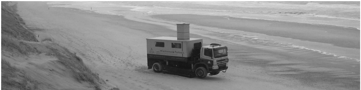
Figure 1. CPT investigation on the beach at the Dutch coast.
