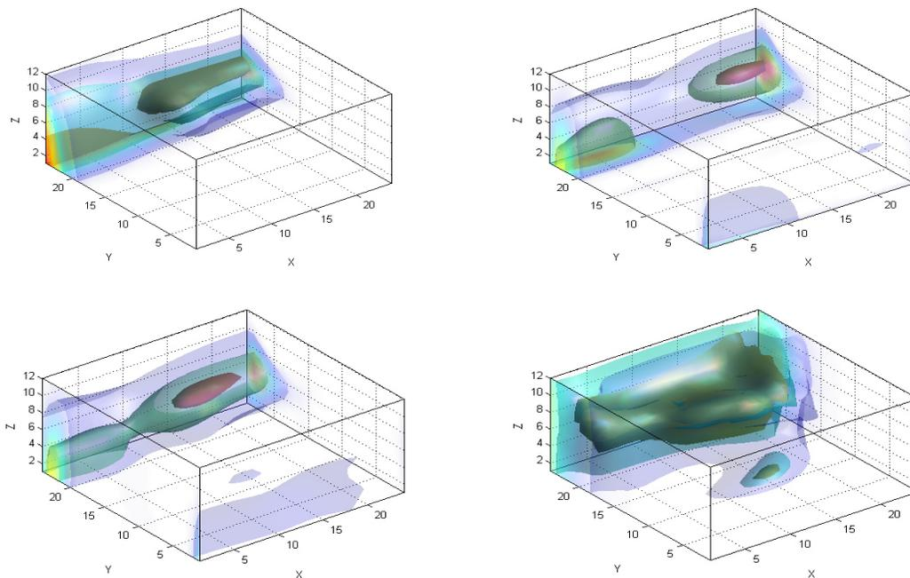
**Figure 3. Upper left: the true initial seawater front shape  $\omega_0$ ; upper right: the estimate of  $\omega_0$  based solely on GW model; left bottom: the result of hydrogeophysical inversion for  $\omega_0$  ; right bottom: EM inversion only for  $\omega_1$ . The level sets of solute fraction:  $\omega = 0.1, 0.4$  and  $0.7$  are displayed (red -  $0.7$  down to light blue -  $0.1$ ).**
