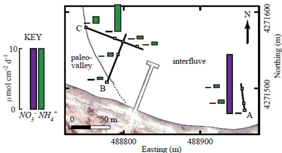
Figure 2. Calculated  $\text{NO}_3^-$  and  $\text{NH}_4^+$  fluxes across the sediment-water interface. Scale bar is shown at left. Fluxes were calculated based on 1-D advection and dispersion calculated from seepage meter measurements and fitted dispersion coefficients for salinity profiles along transects A-A', B-B', and C-C'. From Sawyer et al., in press.
