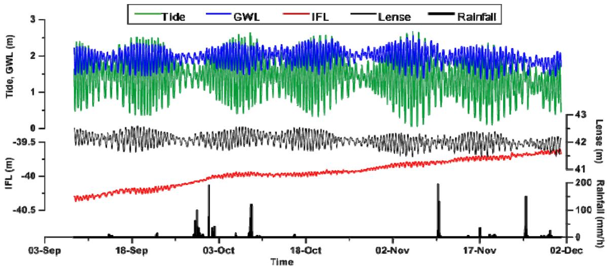
Figure 2. Time series data of groundwater and interface levels
