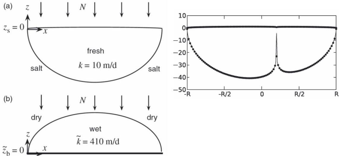
**Figure 1. (a) Cross section of unconfined interface flow on a circular island, (b) equivalent unconfined flow problem in transformed model domain (vertical exaggeration much larger in bottom figure than in top figure). On the right: comparison of Strack solution (line) with MODFLOW (dots) for the simulation with a pumping well (200 m from center island, radius 0.3 m and discharge 200m<sup>3</sup>/d).**
