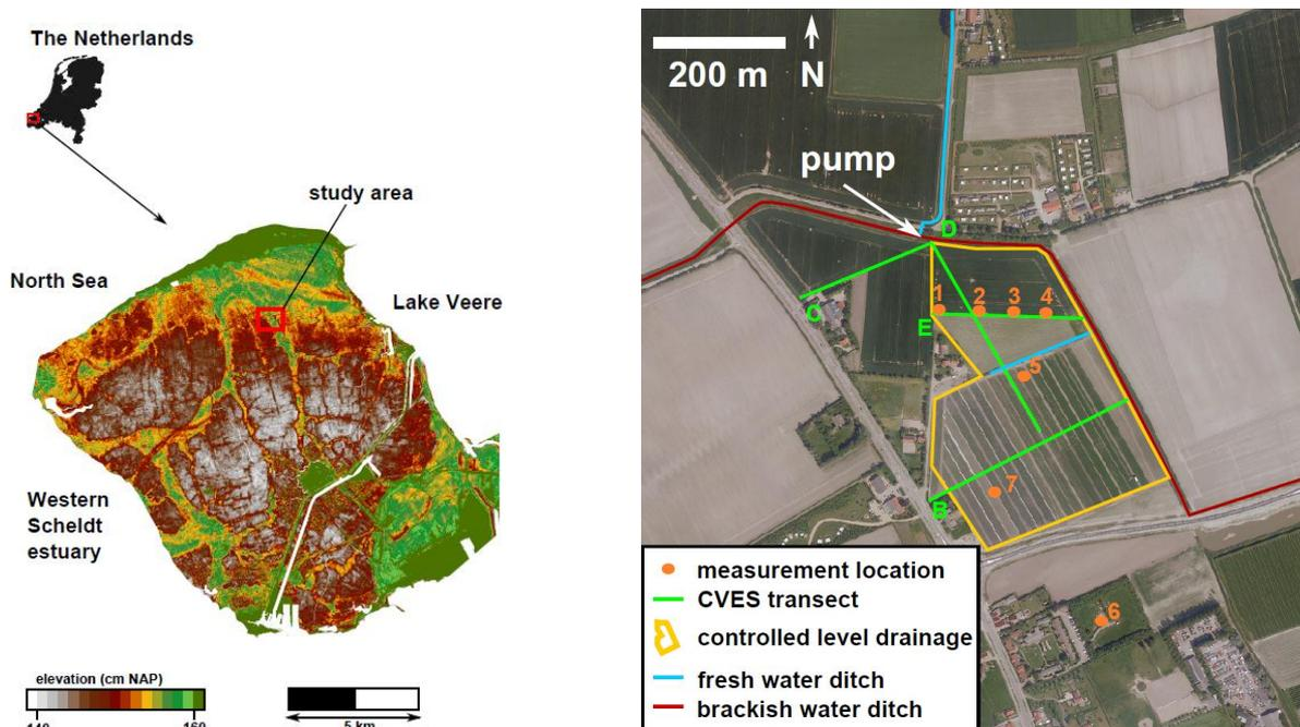
Figure 2: Left: Study area where the controlled level drainage has been installed. Right: Overview of the controlled level drainage area, the most relevant brackish and fresh water ditches and the measurement locations.
