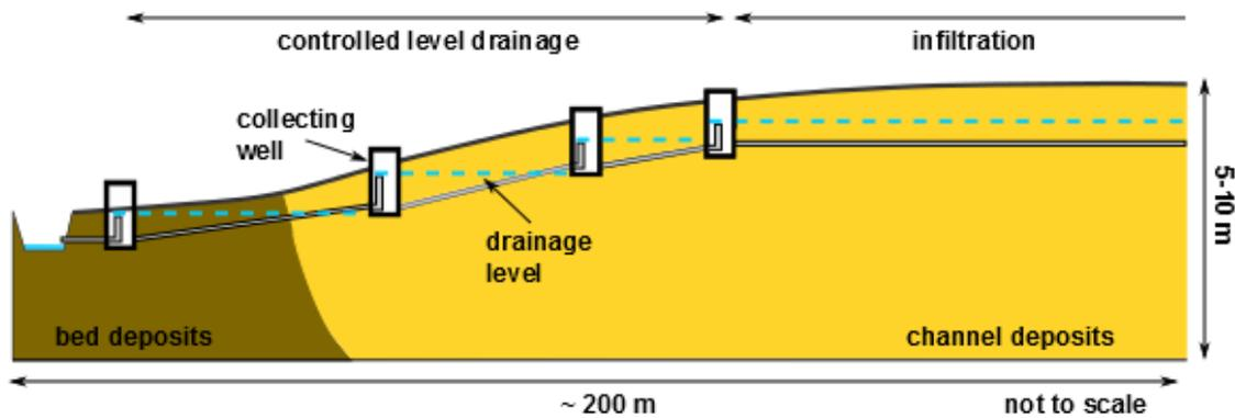
Figure 1: concept of controlled level drainage in a creek ridge.
