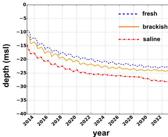
**Figure 4: Result of the numerical model which was used to estimate the long-term effect of the measure. The blue, orange and red lines indicate the 1000, 5000 and 10000 mg l<sup>-1</sup> Chloride contour. Chloride is used as a representative proxy and varies between 0 (fresh water) and 18630 mg l<sup>-1</sup> (sea water).**
