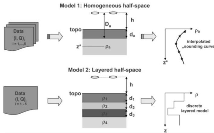
**Figure 2. HEM inversion scheme based on the model of a homogeneous half-space and of a layered half-space model (Siemon and Steuer 2011).**
