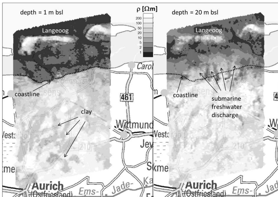
**Figure 3. HEM resistivity maps at 1 and 20 m bsl plotted on a topographic map (BKG 2014). Dark colours indicate conductive areas, like saltwater. White colours indicate more resistive areas, like freshwater saturated sandy sediments.**
