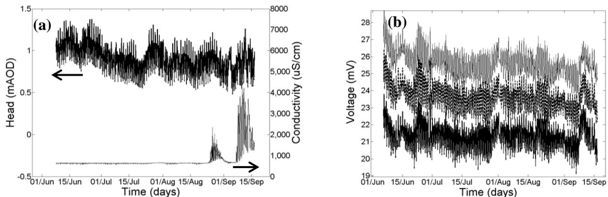
**Figure 1 (a) Head and conductivity measured in the borehole. (b) The voltage measured in the borehole at -26.81mAOD, -14.81mAOD and -2.81mAOD. There is a gradient with depth with the voltage decreasing at the shallower electrodes.**
