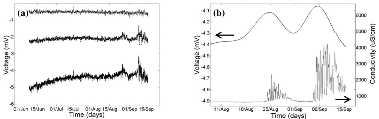
**Figure 2 (a) Voltage at  $-26.81\text{mAOD}$ ,  $-14.81\text{mAOD}$  and  $-4.81\text{mAOD}$  and referenced against the electrode at  $-2.81\text{mAOD}$ . (b) Filtered voltage and FEC at  $-26.81\text{mAOD}$  showing an increase in voltage prior to breakthrough of saline water.**
