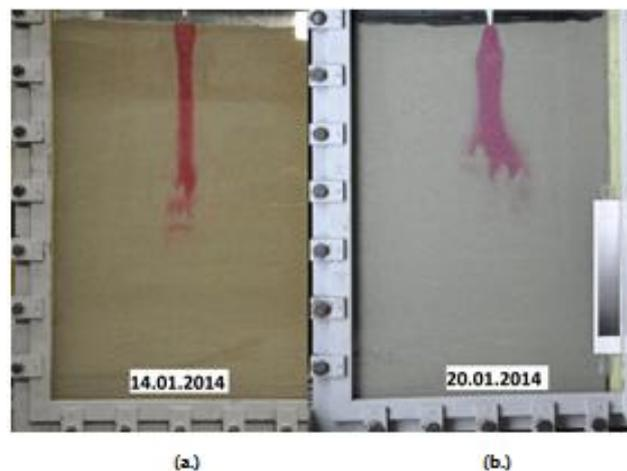
**Figure 2. Results of the variable-density flow experiment at  $t = 15$  min with an infiltration rate of 12.5 ml/min. The source is located (a) ca. 10 cm above the porous medium, and (b) within the porous medium**
