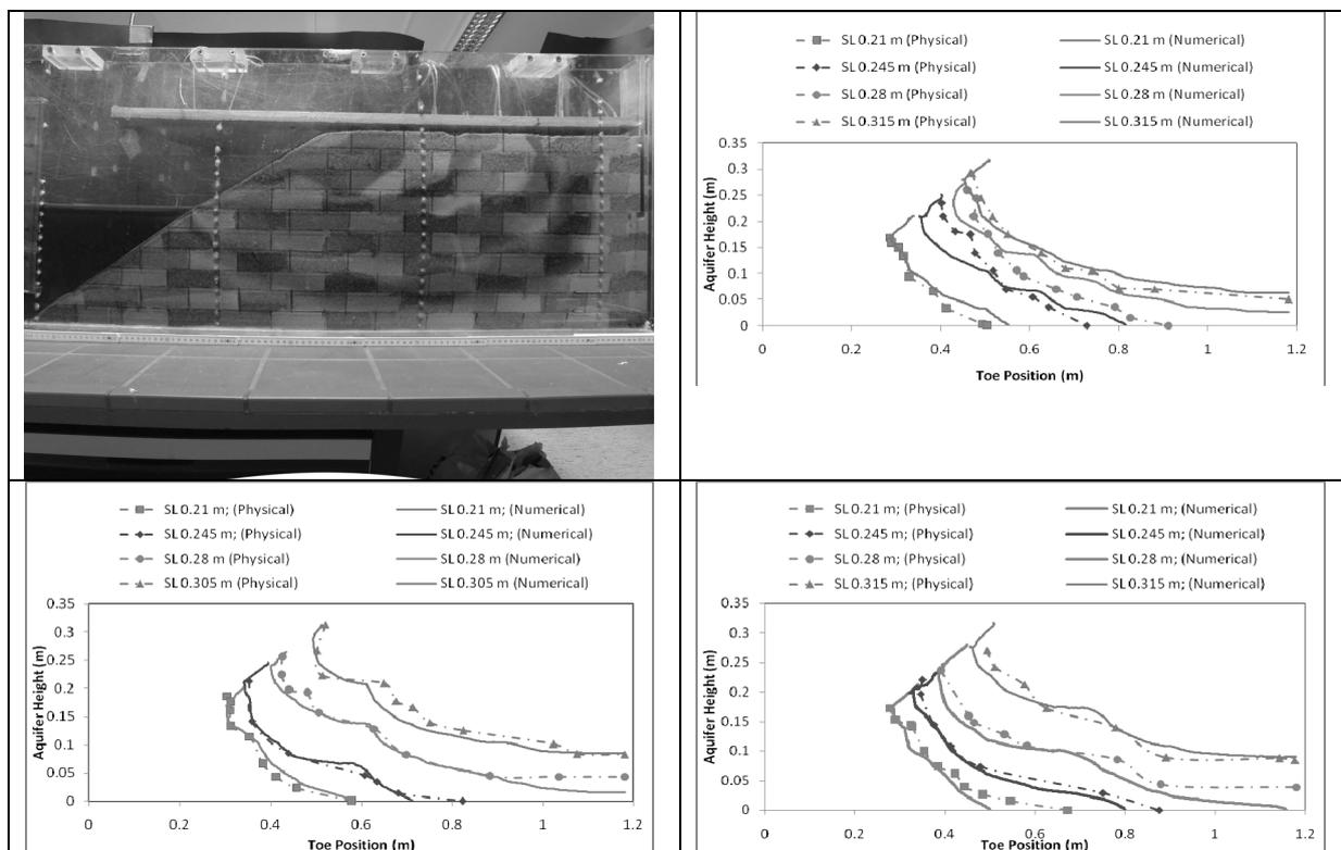
**Figure 1: SFI geometry as a function of compartment length and for different sea levels in a) physical model with a compartment length of 9 cm (Experiment 1); results: b) Experiment 1 (compartment length 9 cm); c) Experiment 2 (18 cm); d) Experiment 3 (27 cm).**
