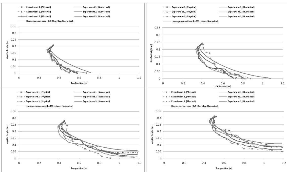
**Figure 2: SFI positions in physical and numerical models as a function of sea level a) sea level 0.210 m, b) 0.245 m, c) 0.280 m, and d) 0.315 m with a constant recharge of 1.73 m/day (a simulated interface geometry of a homogeneous case is also included, orange curve)**
