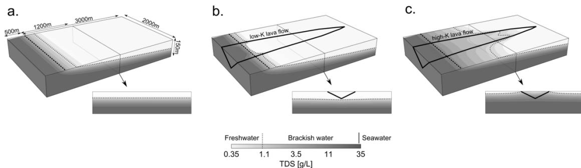
**Figure 2 : Role of local heterogeneities on seawater intrusion in the coastal zone: (a) homogeneous model; (b) palaeovalley infilled with lower permeability (K) lava flow; (c) palaeovalley infilled with higher permeability lava flow. The top face is at mean sea level elevation. Dashed line is the coastline and dotted line is the contour 1 g/L corresponding to the WHO (2003) max salinity standard for drinking water. Vertical exaggeration x3.**
