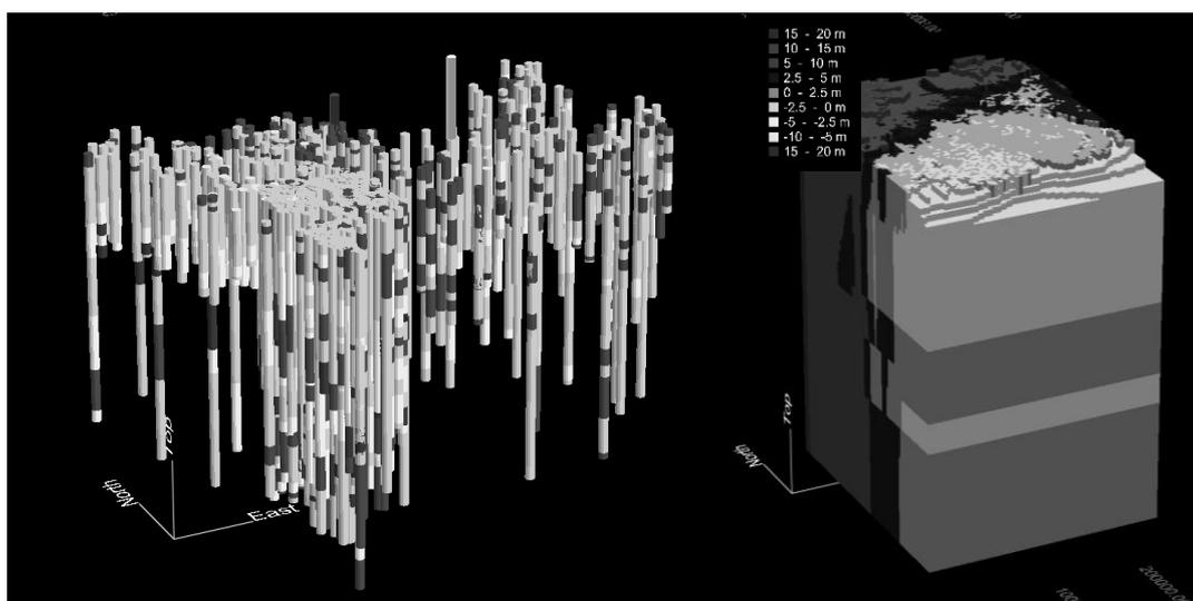
**Figure 3: 3D images of the input data for the model visualized and managed with iMOD-SEAWAT. a: 3D visualization of the collected borehole dataset. b: Point water heads in a subdomain of the modeled area.**
