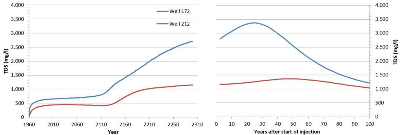
**Figure 3. Effect of injection wells on TDS concentration in two groundwater abstraction wells. Location of wells, see figure 1. Left panel shows effects of a climate scenario implemented from year 2011. Right panel shows effect on TDS concentrations of 100 years water injection starting in the year 2300.**
