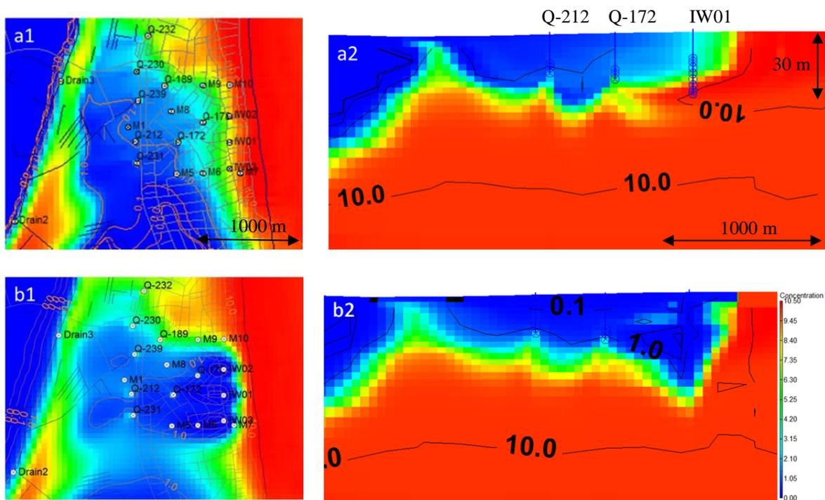
**Figure 2. Saltwater distribution, plan view and cross section. Plan view: model layer 8, elevation -22m. Cross sections through wells Q-212, Q-172, and IW01. Panel a1 and a2: before injection. Panel b1 and b2: after 100 years injection. Contours: TDS (g/l).**
