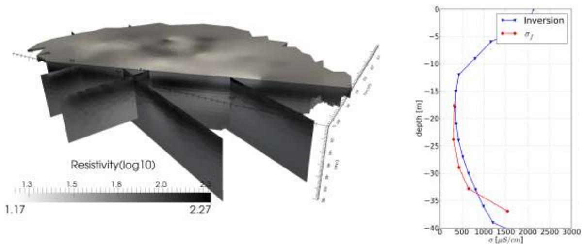
**Fig. 2: 3D inversion result of test site Müllrose together with 2D ERT results (left) and measured fluid conductivities together with fluid conductivities derived from the LE-ERT result using a fitted Waxman-Smiths equation.**
