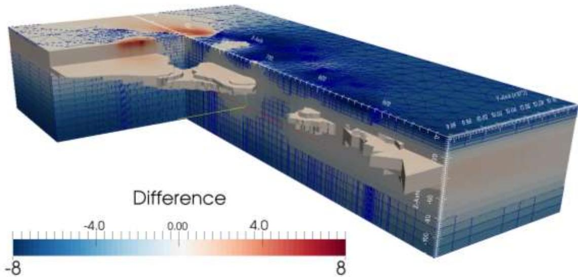
**Fig. 3: Difference (in per cent) between two time steps (June and September) from monitoring measurements of the test site Müllrose. Cells with edges indicate decreasing resistivity and the cells without edges denote increasing resistivity.**
