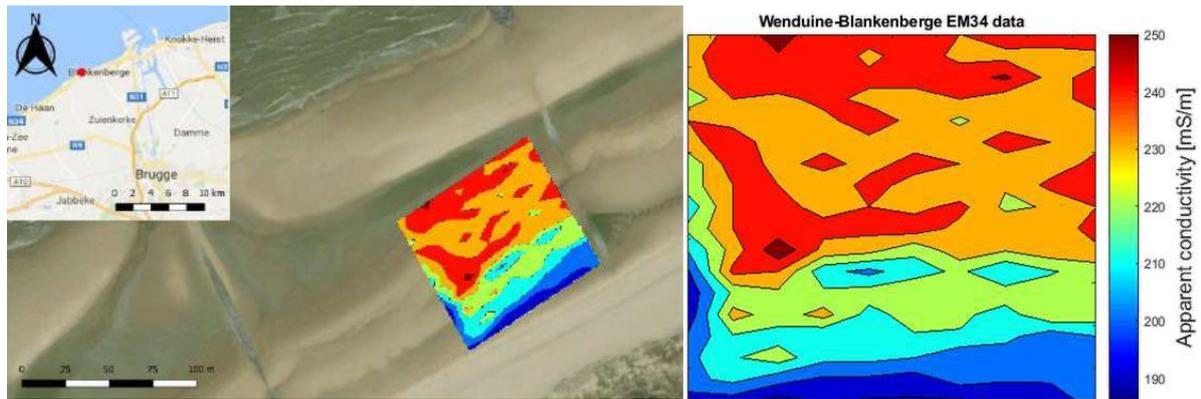
**Figure 1. The first results of mapping with the EM34 device in the Wenduine area. The data was acquired on 14th February 2018 using the EM34 with horizontal dipole and a spacing of 10 m (frequency of 6.4 kHz), which gives an approximated depth of around 7.5 m.**
