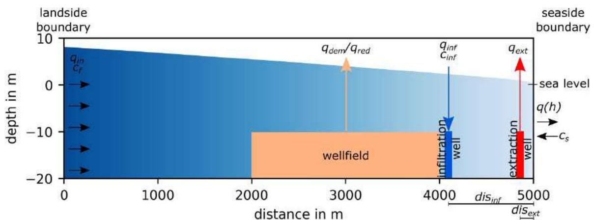
Figure 1. Conceptual model and varied management parameters,  $q_{dem}/q_{red}$  – abstractions to meet the regional water demand,  $q_{ext}$  – extraction rate,  $q_{inf}$  – infiltration rate,  $c_{inf}$  – infiltration concentration,  $dis_{ext}$  – distance to coast of the extraction barrier,  $dis_{inf}$  – distance to coast of the infiltration barrier.
